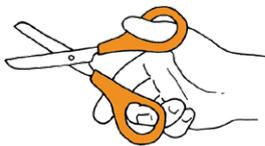
The most ergonomic way to hold scissors is to put the thumb through the upper grip hole and the middle finger through the lower hole - or both the middle and ring finger through the lower hole if it's big enough. The index finger is placed beneath the underside of the lower handle, giving greater stability and allowing you to cut in a straight line.
